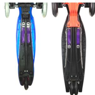
3. Next peel off the plastic backing on the strip of LED lights, to reveal the adhesive strip and carefully stick these along the inside edge of the deck (see Picture 3) so that the LED lights are facing out sideways from the scooter.
